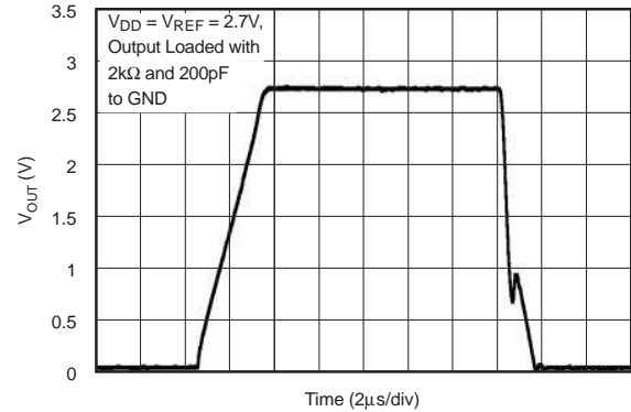
Figure 21. Full-Scale Settling Time (Large Signal)
