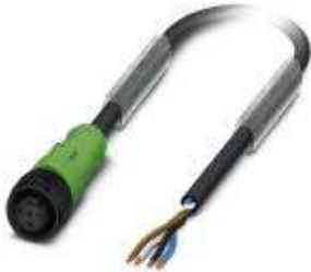
Sensor/Actuator cable, 4-position, PUR halogen-free, Black-gray RAL 7021, Free cable end, on Socket straight M12, A-coded, Cable length: 5 m, with plastic knurl
