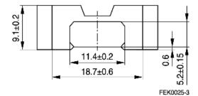
Material  $P_V$ A<sub>I</sub> value Ordering code  $\mu_e$ nΗ W/set 900 +30/-20% PC200<sup>1)</sup> < 1.2 ( 50 mT, 1000 kHz, 100 °C) 700 B66421G0000X608 < 1.6 ( 30 mT, 2000 kHz, 100 °C) 2000 +30/-20% N87 1560 < 1.8 (200 mT, 100 kHz, 100 °C) B66421G0000X187 **N97** 2100 +30/-20% 1640 < 1.5 (200 mT, 100 kHz, 100 °C) B66421G0000X197
