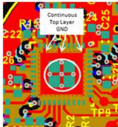
Figure 14. Continuous GND Layout
