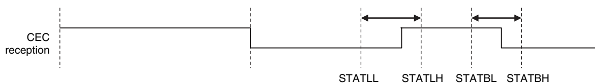
Figure 13-42. Start Bit Reception Timing
