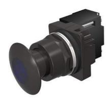
30mm BlackMax, Epoxy Coated Corrosion Resistant Complete Metal Unit Illuminated Push-Pull Operator Transformer type, 120V AC LED Lamp Mushroom Head Cap Small 1 3/4" (44.5 mm) Metal, Black with Blue Lens 2 Position Maintained, Pull-to-Release UL Listed, CSA Certified NEMA 1,3,3R,4,4X,12,13 & Automotive Standards
