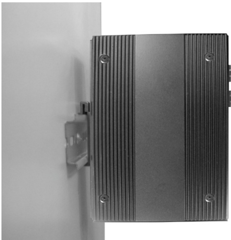
Figure 2.7: Installation to DIN-rail Step 2
