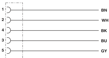
Contact assignment of the M12 socket
