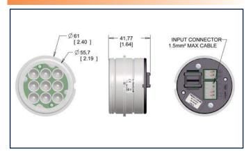
Diameter x H 61mm x 41.8mm (2.40" x 1.65") Maximum Cable Dia - 1.5mm<sup>2</sup> / 16 AWG
