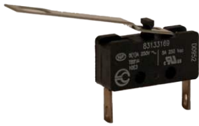
Maintained action variant (bistable reset switch) for level regulation. Has lever with hole for push-pull actuation by a rod with 2 stops
