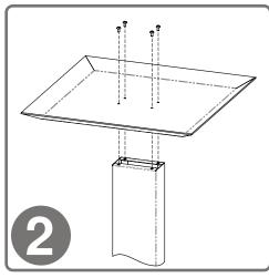
Use Phillips screwdriver to secure base to column with (4x) screws  $(10-32 \times 5/16")$ .
