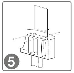
To mount the MP-070 Sign Holder, place the lip of the holder over the front edge of the dispenser, lining up holes. With a flathead screwdriver, attach using (2x) barrel screws included with sign holder.
