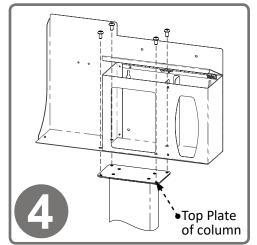
Attach the RS005-0412 Respiratory Hygiene Station to the column using (4x) screws included with stand. One pair of screw holes is located in the hand sanitizer dispener section; the second pair are inside the facemask section and can be accessed with the lid open. Tighten all screws.
