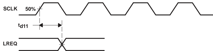
Figure 6-7. TSB12C01A Link-Request-to-Phy-Layer Waveforms
