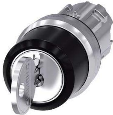
RONIS key-operated switch, 22 mm, round, metal, shiny, lock number SB30, with 2 keys, 3 switch positions I>O<II, momentary contact on the left, latching on the right, actuating angle 2x45°, 10:30h/12h/13:30h, Key removal O+II, possible special locks: SB31, 421, 455, Z=50-unit packaging
