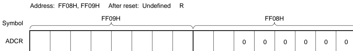
Figure 10-6. Format of A/D Conversion Result Register (ADCR)
