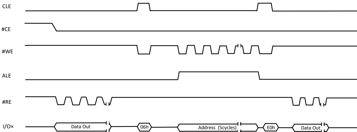
Figure 9-4 Two Plane Random Data Read (06h-E0h) Operation
