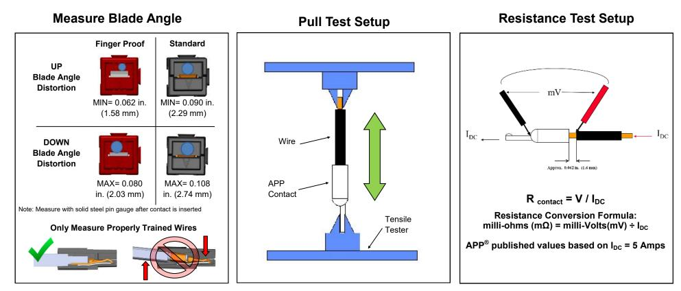
The included crimp performance and dimensional information are provided as a means to verify quality crimping of Anderson Power Products® contacts and is based on the use of tooling. The assembly of connector solutions with tooling assures that all crimp performance and fit specifications are met. Customers must regularly re-check electrical performance and dimensions of crimps to determine if crimp tools require maintenance due to wear over time.
