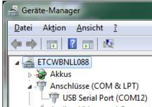
Figure 11: The Demo Kit must be visible as a virtual ComPort in the Windows device manager.
