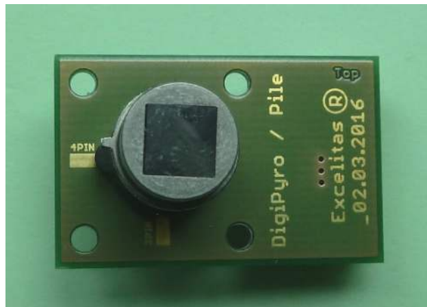
Figure 8: Alignment of TO housing nose with the marking on the board.
