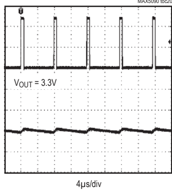
A: SWITCH VOLTAGE (LX PIN), 20mV/div ( V_{IN} = 48V ) B: INDUCTOR CURRENT, 2A/div ( I_0 = 2A )
