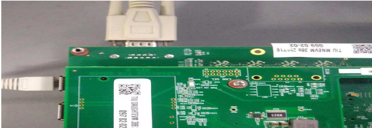
Figure 8. Connecting to Console Window
