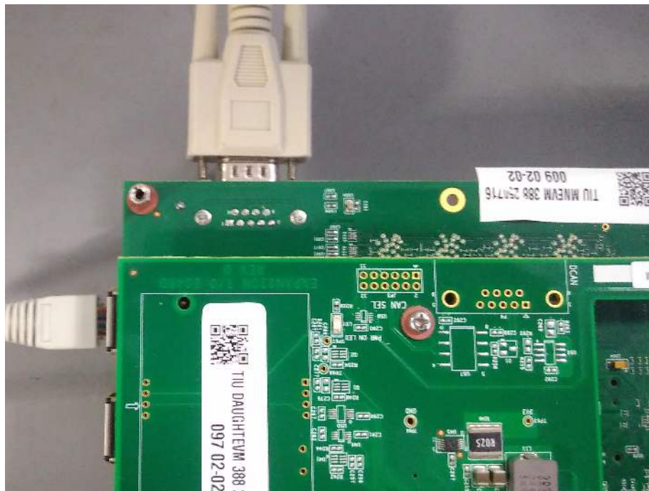
Figure 7. Serial Cable Connected to EVM
