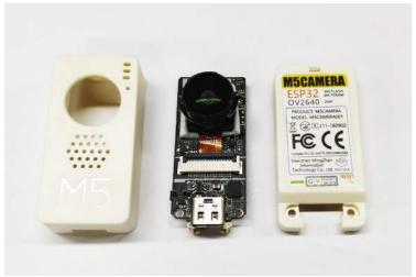
The hardware comes preloaded software, programmed by ESP-IDF. It is an application to run Wi-Fi camera. The output image is size 600\*800, since it's 2-Maga camera, you sure can optimize the software to output the maximum size of photos.
