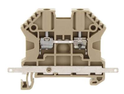
Feed-through terminal, Screw connection, Mounting type: Mounting rail TS 35/7.5, Rated cross-section: 2.5 mm², Width: 5 mm, Colour: White
