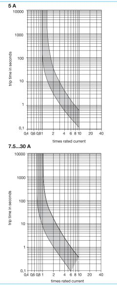
The time/current characteristic curve depends on the ambient temperature prevailing. In order to eliminate nuisance tripping, please multiply the circuit breaker current ratings by the derating factor shown below. See also section Technical information.
