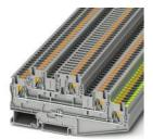
Disconnect terminal block, Current and voltage are determined by the plug used., nom. voltage: 500 V, nominal current: 30 A, number of connections: 5, connection method: Push-in connection, Rated cross section: 4 mm<sup>2</sup>, cross section: 0.2 mm<sup>2</sup> - 6 mm<sup>2</sup>, connection method: Push-in connection, Rated cross section: 4 mm<sup>2</sup>, cross section: 0.2 mm<sup>2</sup> - 6 mm<sup>2</sup>, mounting type: NS 35/7,5, NS 35/15, color: gray
