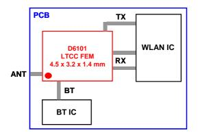
The D6101 front-end module is intended for mobile phone applications, where size is a critical parameter.
