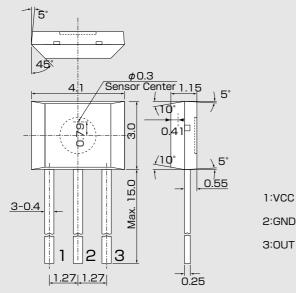
Note 1) The sensor center is located within the  $\phi$ 0.3mm circle.
