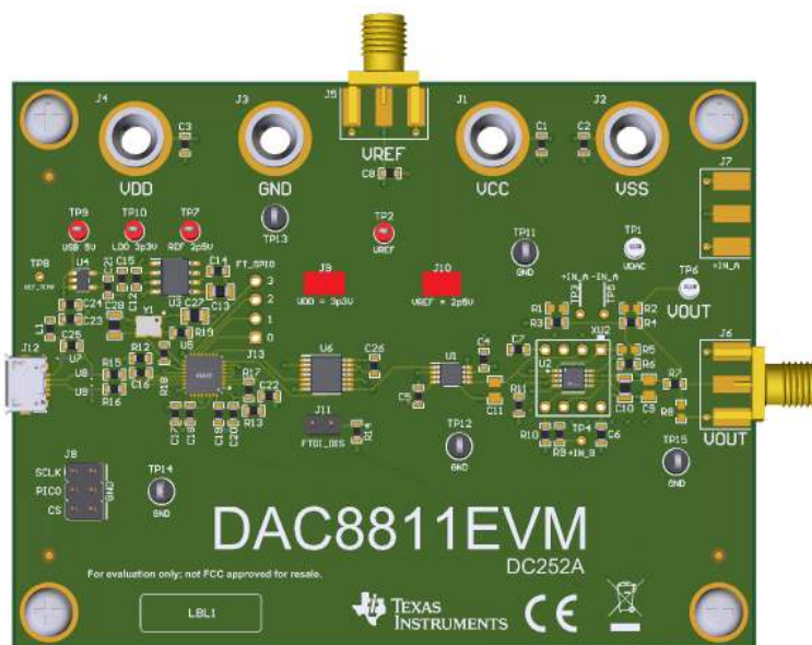
Figure 2-1. Default Header Settings for the DAC8811EVM
