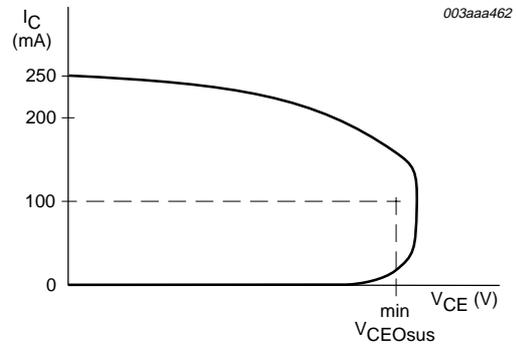
**Fig 10. Oscilloscope display for collector-emitter sustaining voltage.**
