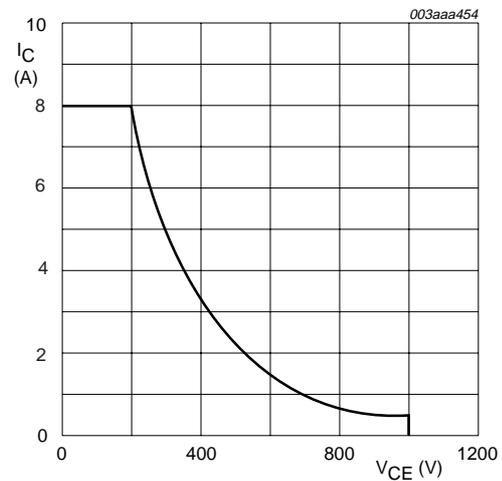
$V_{BE} = -1 \text{ V to } -5 \text{ V}; T_h = 100^\circ \text{C}.$
