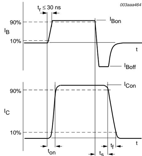
**Fig 12. Switching time waveforms with resistive load.**
