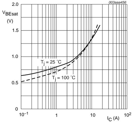
$T_j = 25\text{ }^\circ\text{C}$  and  $100\text{ }^\circ\text{C}$
