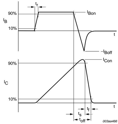
**Fig 14. Switching time waveforms with inductive load.**
