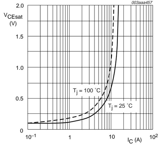
$T_j = 25\text{ }^\circ\text{C}$  and  $100\text{ }^\circ\text{C}$
