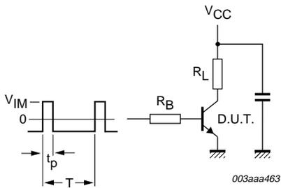
$V_{CC} = 250\text{ V}$ ;  $t_p = 20\ \mu\text{s}$ ;  $V_{IM} = -6\text{ V to } 8\text{ V}$ ;  $t_p/T = 0.01$ .
