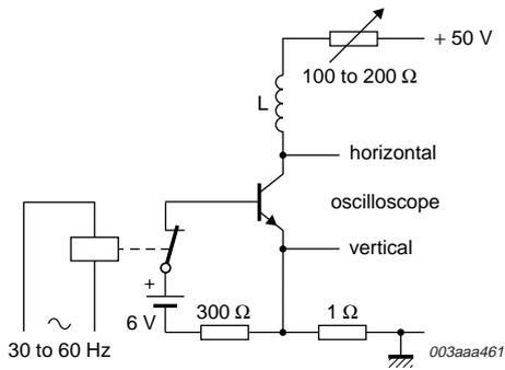
**Fig 9. Test circuit for collector-emitter sustaining voltage.**
