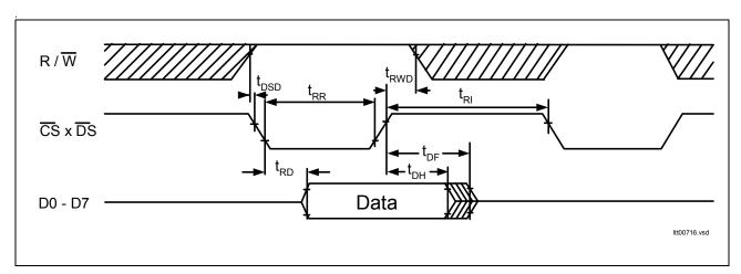
Figure 69 Microprocessor Read Timing
