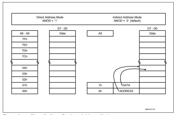
Figure 8 Direct/Indirect Register Address Mode
