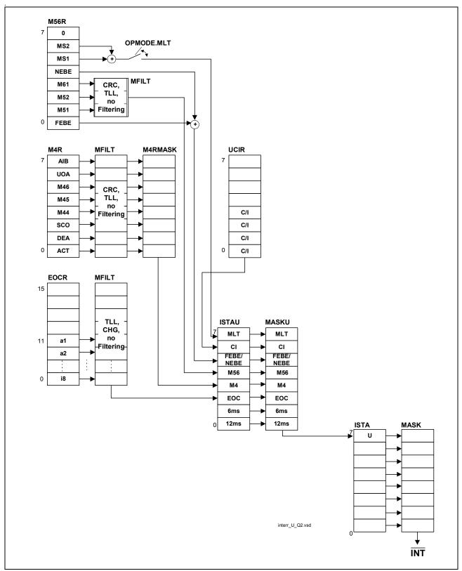
Figure 77 Interrupt Structure U-Transceiver Q-SMINT®I: 2B1Q
