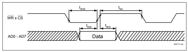
Figure 66 Microprocessor Write Cycle
