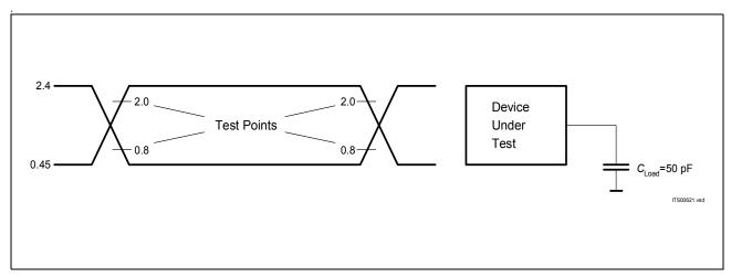
Figure 61 Input/Output Waveform for AC Tests
