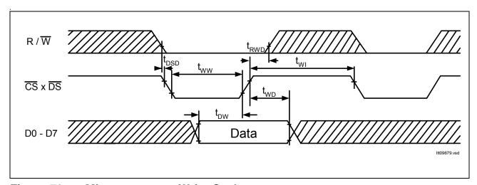
Figure 70 Microprocessor Write Cycle
