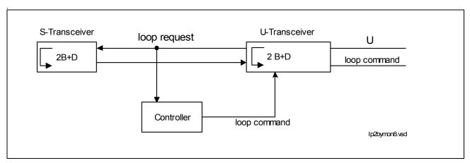
Figure 51 Complete Loopback Options in NT-Mode
