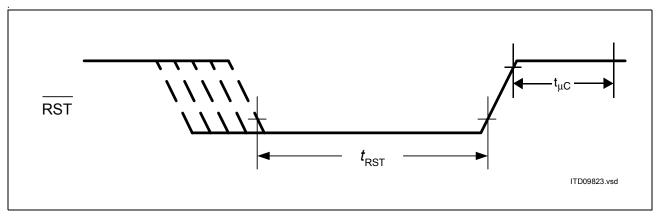
Figure 72 Reset Input Signal
