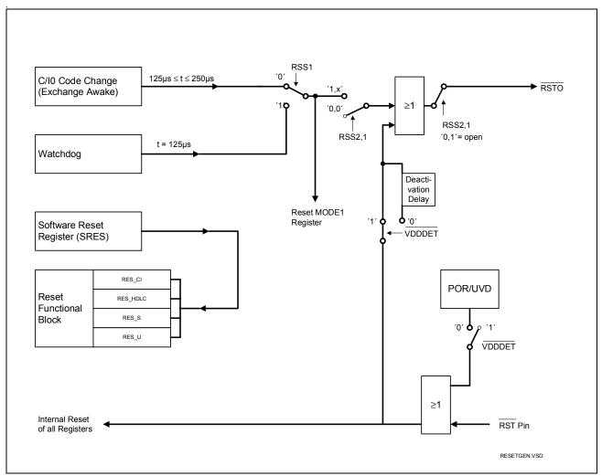
Figure 9 Reset Generation of the T-SMINT®I<sup>1)</sup>
