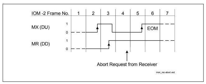
Figure 21 Monitor Channel, Transmission Abort requested by the Receiver
