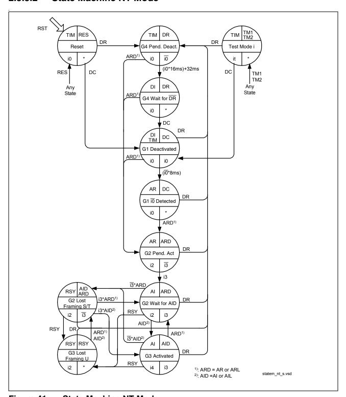
Figure 41 State Machine NT Mode
