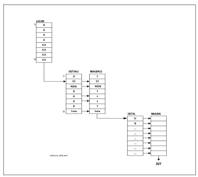
Figure 36 Interrupt Structure U-Transceiver
