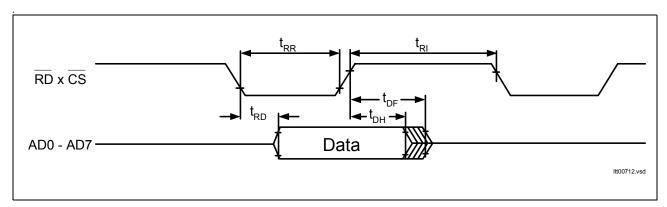
Figure 65 Microprocessor Read Cycle
