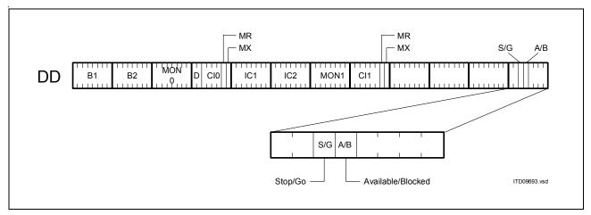
Figure 29 Structure of Last Octet of Ch2 on DD
