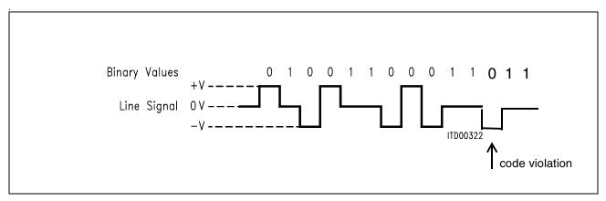
Figure 37 S/T -Interface Line Code
