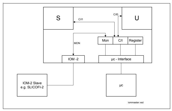
Figure 4 Control via µP Interface
