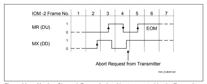
Figure 22 Monitor Channel, Transmission Abort requested by the Transmitter
