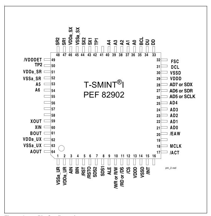
Figure 1 Pin Configuration
