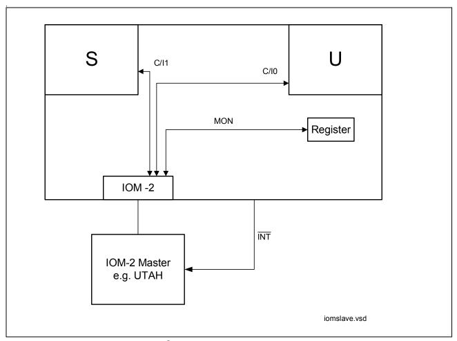
Figure 5 Control via IOM®-2 Interface
