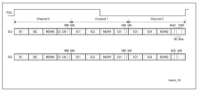
Figure 10 IOM®-2 Frame Structure of the T-SMINT®I
