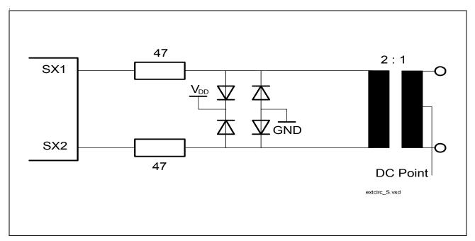
Figure 55 External Circuitry S-Interface Transmitter
