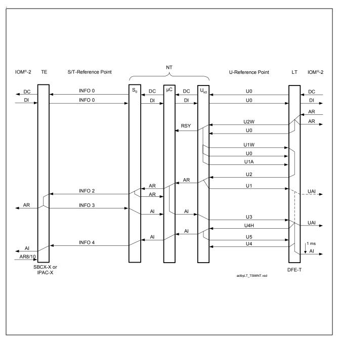
Figure 44 Activation Initiated by Exchange
