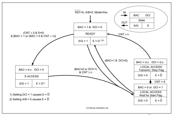
Figure 30 State Machine of the D-Channel Arbiter (Simplified View)<sup>1)</sup>
