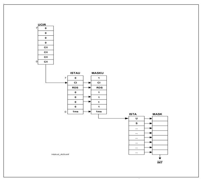
Figure 78 Interrupt Structure U-Transceiver T-SMINT®I: 4B3T
