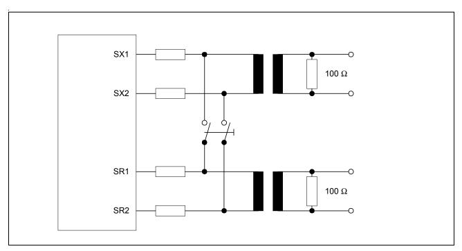
Figure 50 External Loop at the S/T-Interface
