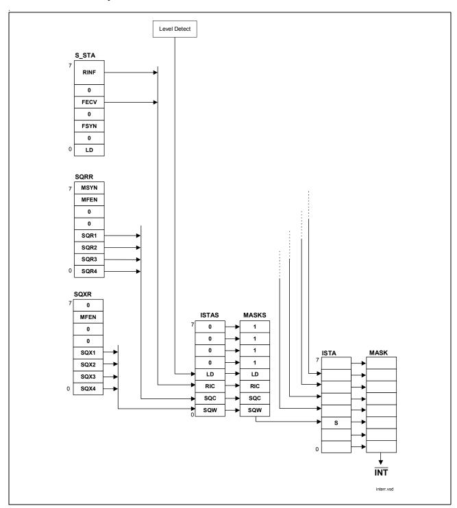
Figure 43 Interrupt Structure S-Transceiver
