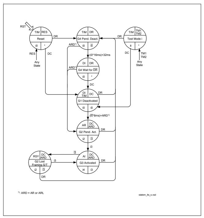
Figure 42 State Machine LT-S Mode
