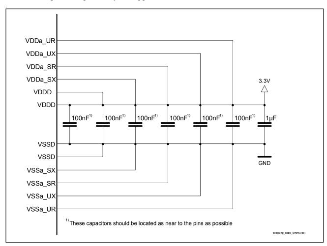
Figure 53 Power Supply Blocking
