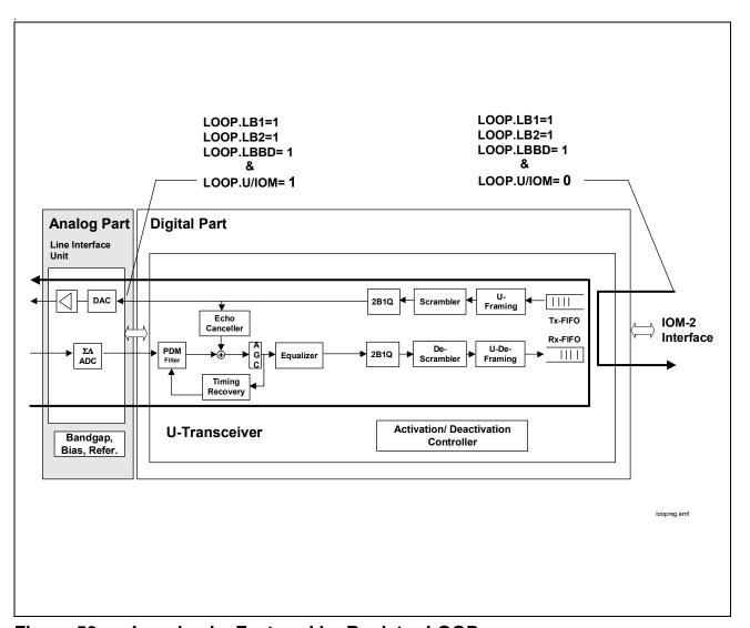
Figure 52 Loopbacks Featured by Register LOOP
