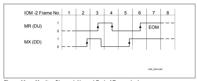
Figure 23 Monitor Channel, Normal End of Transmission
