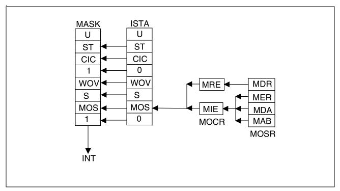
Figure 24 MONITOR Interrupt Structure
