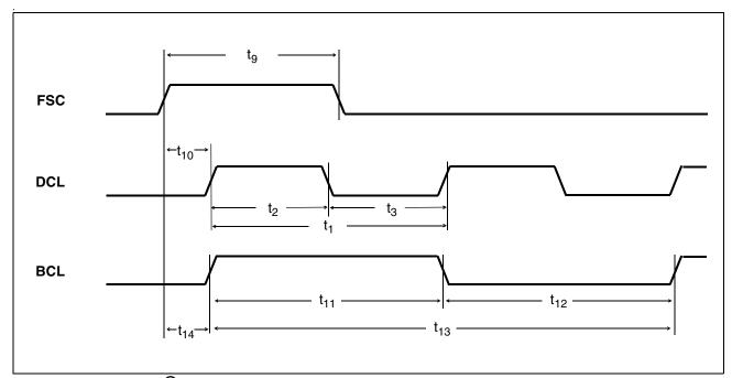
Figure 63 IOM<sup>®</sup>-2 Interface - Frame Synchronization Timing
