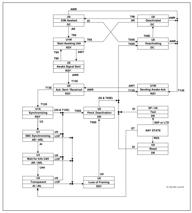
Figure 35 NT State Machine (IEC-T/NTC-T Compatible)
