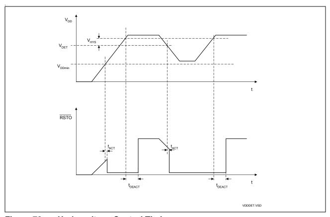
Figure 73 Undervoltage Control Timing
