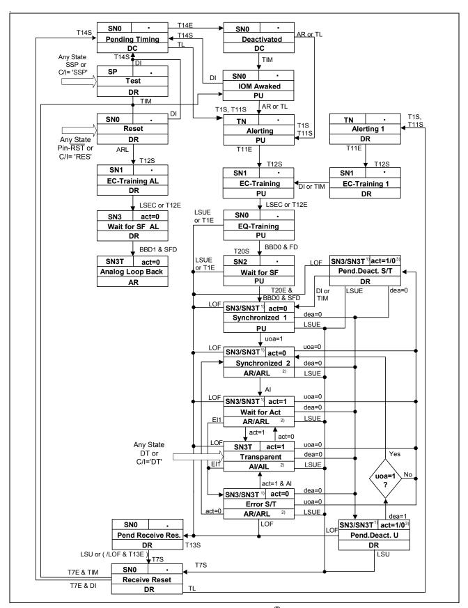
Figure 75 Simplified State Machine Q-SMINT®I: 2B1Q
