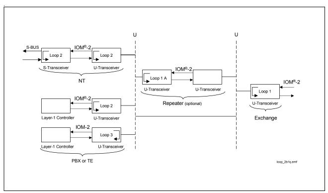
Figure 49 Test Loopbacks
