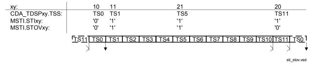
Figure 18 Examples for the Synchronous Transfer Interrupt Control with one STlxy enabled
