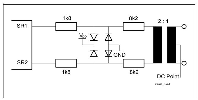
Figure 56 External Circuitry S-Interface Receiver
