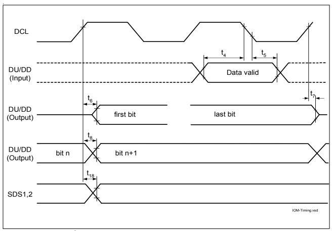
Figure 62 IOM®-2 Interface - Bit Synchronization Timing
