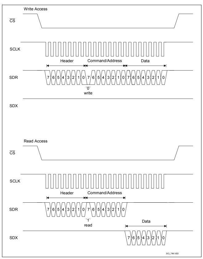
Figure 6 Serial Control Interface Timing
