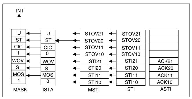
Figure 17 Interrupt Structure of the Synchronous Data Transfer
