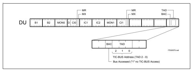
Figure 28 Structure of Last Octet of Ch2 on DU
