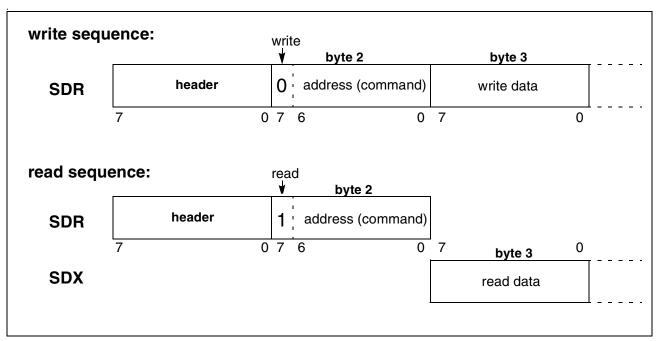
Figure 7 Serial Command Structure
