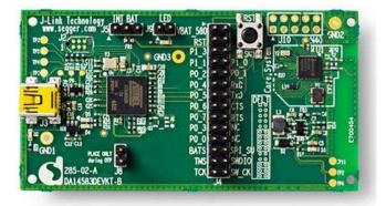
This Basic development kit gives you all flexibility to develop with confidence. All of the DA14583's I/Os are available and mapped on to expansion connectors. A debugger is provided on the PCB which in combination with SmartSnippets<sup>™</sup>, Dialog's complete software environment, enables you to program and test your Bluetooth Smart application.
