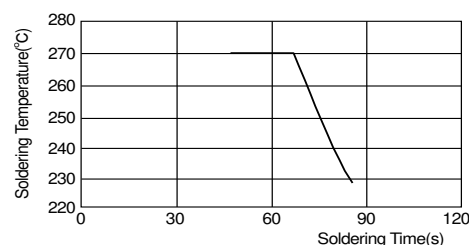
[Allowable Reflow Soldering Temperature and Time]
