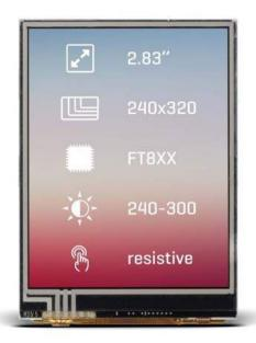
The **240x320px** screen is driven by an **FT800** graphic controller which is supported in <u>Visual</u> <u>TFT</u>, the GUI design tool for rapid development of user interfaces.
