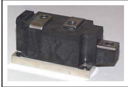
ND41__35 Dual Diode Isolated POW-R-BLOK™ Module 350 Amperes / 600-1700 Volts
