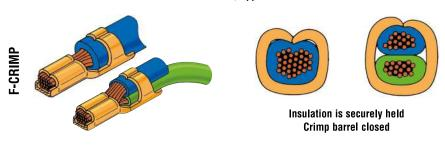
For double wire applications with different size wires always place wire with smallest outer diameter in the bottom
