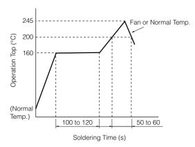
\*Reflow temperature may vary by location even in the same reflow condition. Please check the reflow temperature at terminals and at the top of a switch to make sure the both temperatures are withiin the specification. If even one of them is out of the specifications, please adjust.
