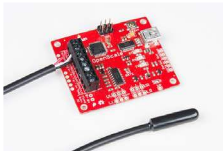
DS18B20 external temperature sensor
