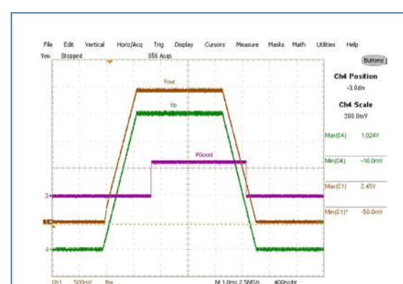
Figure 44: Voltage tracking using Vp pin Ch 1 :Vout, Ch 3 :P Good , Ch 4 :V p
