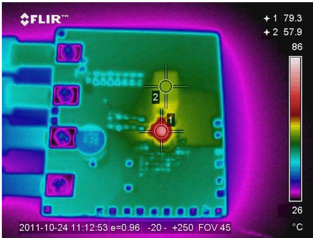
Figure 46: Thermal Image of the Board at 12A Load, Test Point 1 is IR3894, Test Point 2 is inductor
