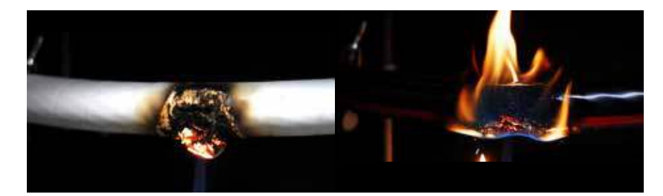
Cable Protected with Scotch® Fire Retardant Electric Arc Proofing Tape 77 During Test
