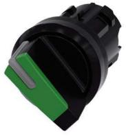
Selector switch, illuminable, 22 mm, round, plastic, green, selector switch, short, 2 switch positions O-I, latching, actuating angle 90°, 10:30h/13:30h Z=50-unit packaging
