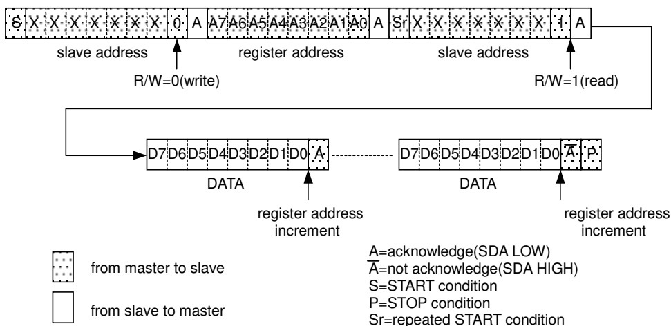
Figure 6. I 2 C Multiple read protocol
