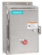
Non-reversing motor starter, Size 3 1/2, Three phase full voltage, Solid-state overload relay, OLR amp range 50-200A, 24VAC 50-60Hz coil, Non-combination type, Encl. type 4X 304 S. Steel, Water/dust tight noncorrosive, Standard width enclosure
