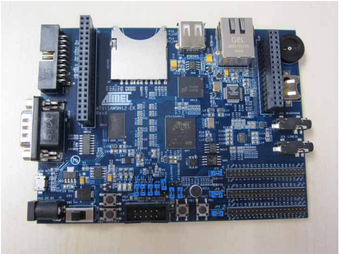
Figure 4-3. SAM9N12-EK Board Layout
