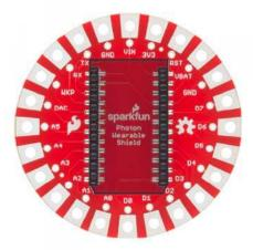
Double check that you put the Photon in the female headers the correct way!
