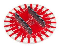
**Please Note:** All SparkFun shields for the Photon are also compatible with the Core from Particle. The WKP, DAC and VBT pins on the Photon will be labeled A7, A6 and 3V3\*, respectively, on the Core, but will not alter the functionality of any of the Shields.
