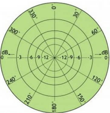
TYPICAL RADIATION PATTERN (H-PLANE)
