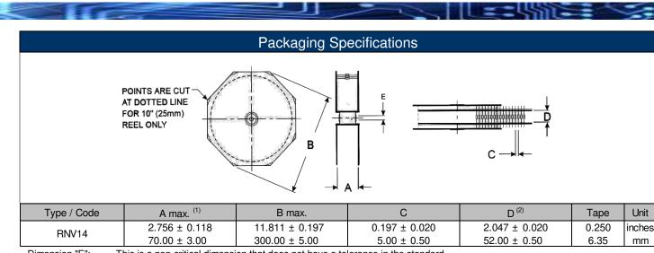
Dimension "E": This is a non-critical dimension that does not have a tolerance in the standard. Range of diameters is from 0.547" (13.9 mm) to 1.5" (38.1 mm)
