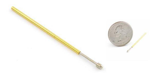
These 33mm (1.3") spring loaded pogo pins are great for programming and applications where you don't always want headers soldered onto your boards. We use them for our programming jigs in production. The pins fit snugly into most standard perf board holes. Solder them just like you would normal wire.
