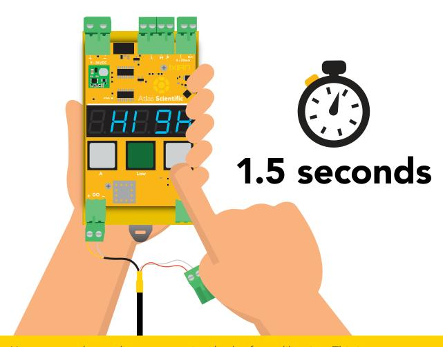
You may see the readings start to rise slowly after calibration. This is not uncommon. Simply press "high" calibration button again. This can be done many times; each time, your calibration will become more accurate. "Prefect Calibration" does not exist. It's is a psychological trap. Limit high point calibration attempts to no more than 10 minutes.
