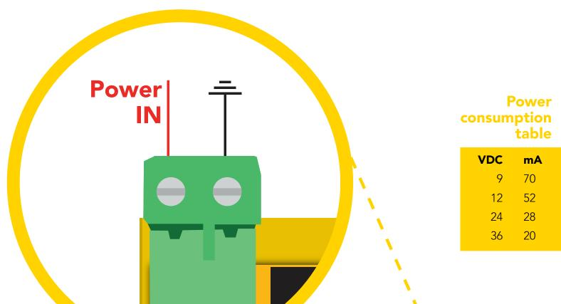
The Industrial Dissolved Oxygen Transmitter must be connected to a power source that provides a smooth, ripple free DC voltage. Any DC power supply designed for a PLC should be sufficient. Connecting this device to a cheap AC adapter also known as a "wall wart" may interfere with the devices ability to provide stable readings .
