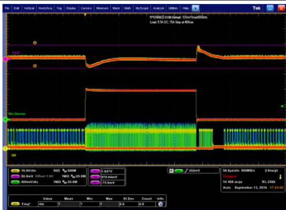
Figure 22. Output Voltage Regulation vs Output Current
