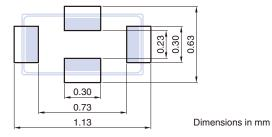
The recommended distance to the PCB ground plane is 0.2mm. Line width should be designed to match  $50\Omega$  characteristic impedance, depending on PCB material and thickness.
