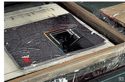
In shrink wrapping operation, 3M™ PTFE Glass Cloth Tape 5451 helps protect the bar underneath where the hot wire seals the plastic film.
