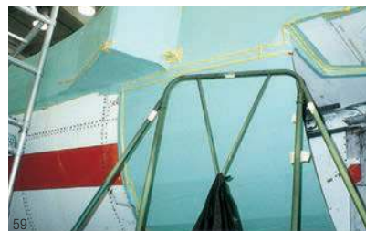
Abrasion-resistant rubber backing and acrylic adhesive of 3M™ Impact Stripping Tapes protect surfaces during plastic media blasting.
