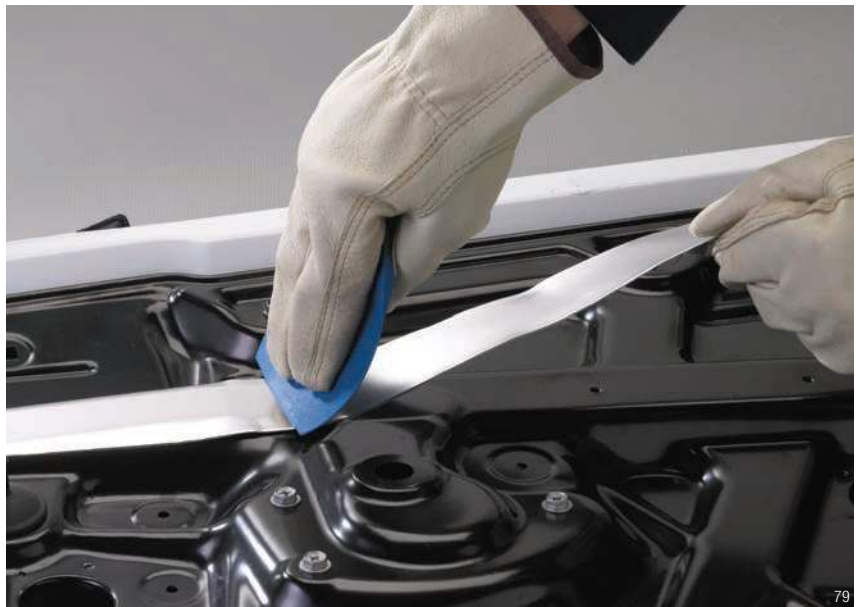
Applied with a 3M™ PA-1 Wiper to the inside of a car door, 3M™ Damping Foil 2552 effectively damps noise and vibration with as little as 10% surface coverage. Optimized acrylic on a dead soft aluminum constraining layer converts vibrational energy to negligible heat that readily dissipates.
