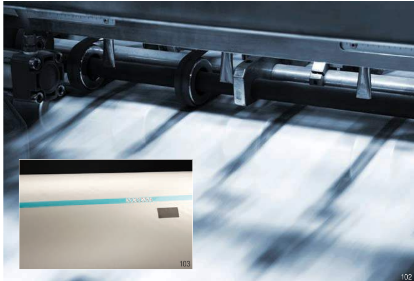
3M™ Repulpable Splittable Flying Splice Tape eliminates the time and work of “V” and “W” patterns with a straight across flying splice. Advanced coating provides a smooth and consistent opening force. A fiber-free break open means less blanket cleanup.
