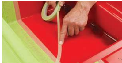
A combination of Scotch® Fine Line Masking Tape and 3M™ Crepe Masking Tape helps to create sharp, high-impact paint lines on an in-mold application in the marine industry.
