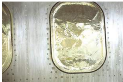
With conformability and chemical resistance, 3M™ Aluminum Foil Tapes used to protect aircraft windows during paint stripping using harsh chemicals.
